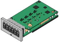
This card provides 6 digital station ports (1-6), 2 analog extension ports (7-8) and 4 analog trunk ports (9-12). The card also includes 10 voice compression channels.
