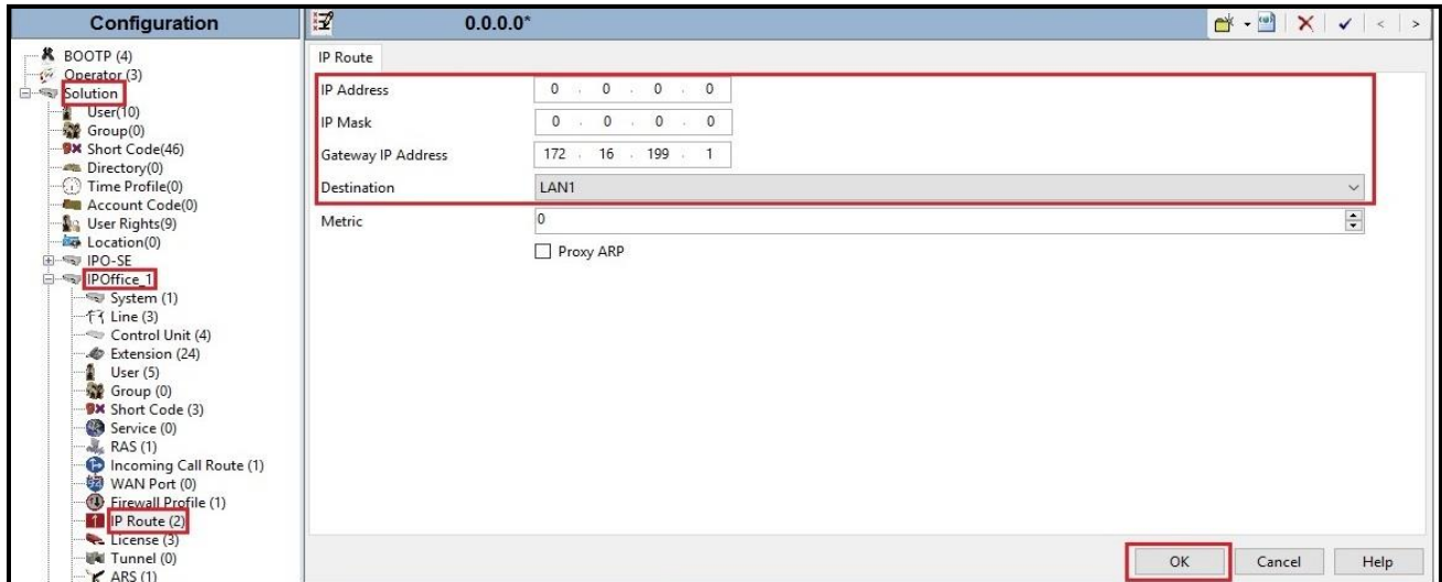
Figure 13 - Avaya IP Office Expansion Server IP Route
