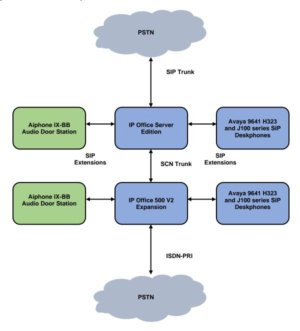
Figure 1: Avaya SIP Telephony Network with Aiphone IX-BB Audio Door Station
