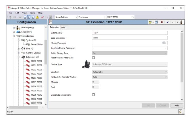
Select the **VoIP** tab and retain the default values. During the compliance test, IX BB was tested with *G.711 ULaw* codec. Enable **Allow Direct Media Path** so that audio/RTP flows directly between two SIP endpoints without using media resources in Avaya IP Office Server Edition. **Media Security** was *disabled* for IX-BB.
