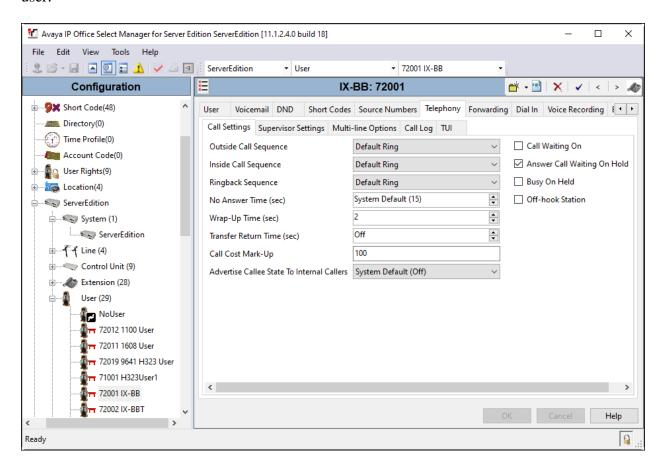
Select the **Supervisor Settings** sub-tab and enter a desired **Login Code**. The **Login Code** is the password that will be used by IX-BB to register with IP Office Server Edition.
