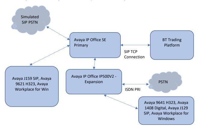
Figure 1: Connection of BT Trading Platform with Avaya IP Office
