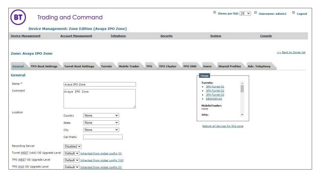
Navigate to the **Turret Boot Settings** tab in Avaya IPO Zone, then select **SIP** option **Basic Mode** (not shown) and update Avaya IP Office server address to 10.128.226.178 and other highlighted parameters below.
