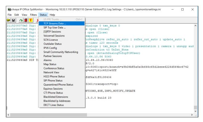
The **TCP Streams** screen is displayed. Verify that there is an entry corresponding to the Shadow CMS server, with the IP address of the Shadow CMS server in the **Dst Addr** column. Also verify that the pertinent entry has the **State** as **Established**.
