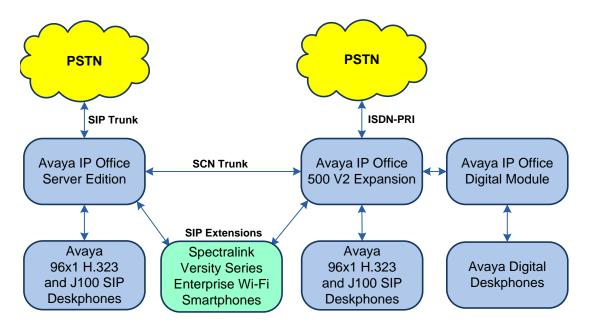
Figure 1: Spectralink Versity 97 Series Enterprise Wi-Fi Smartphones with Avaya IP Office
