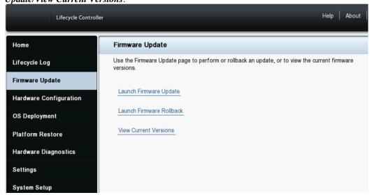
11. Verify versions: BIOS = 2.13.3, Broadcom Gigabit Ethernet = 21.81.3, Integrated Remote Access Controller (IDRAC) = 5.10.00.00, and Lifecycle Controller = 5.10.00.00, Intel Gigabit 4P I350-t rNDC = 20.5.13 and PERC H730P Mini = 25.5.9.0001. Additional packages (i.e. OS Collector 14G, System CPLD, etc.) may update also depending on the vintage of server being updated.
