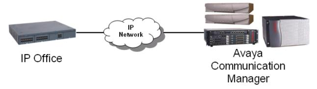
Figure 12: VoIP networking using H.323
