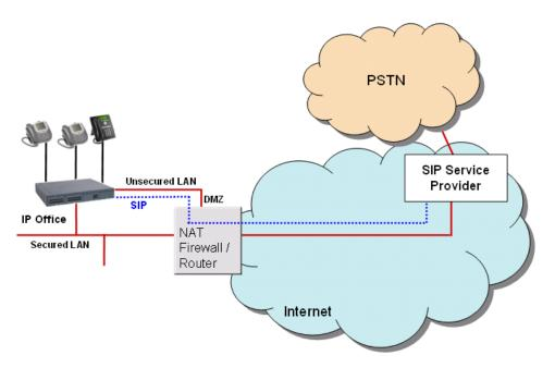
Figure 18: Direct connection from the second Ethernet port to the internet through a DMZ port on the router
