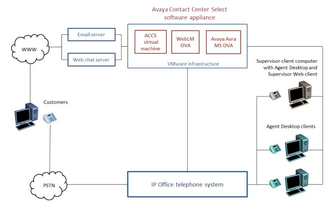
Figure 9: Typical Avaya Contact Center Select and VMware solution
