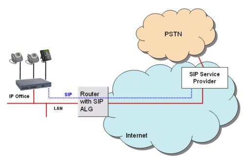
Figure 20: Connection to ITSP through router with ALG to resolves NAT issues
