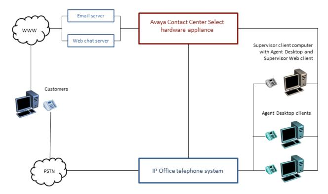
Figure 10: Typical Avaya Contact Center Select hardware appliance solution
