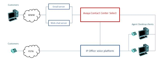
Figure 6: Typical contact center solution using voice and multimedia Avaya Contact Center Select and the Avaya IP Office voice phone system
