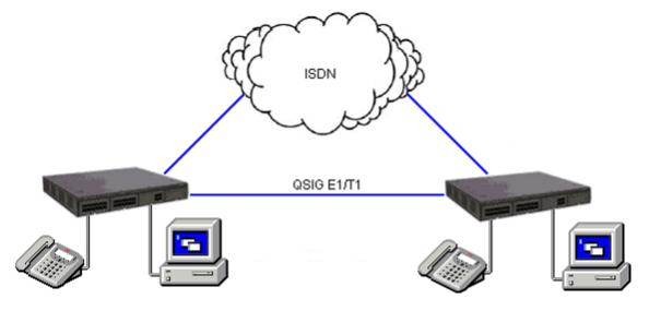
Figure 14: Circuit switched voice networking
