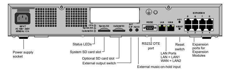
Figure 3: IP500V2 rear view
