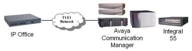
Figure 13: Q.SIG networking using T1/E1 links (TDM)
